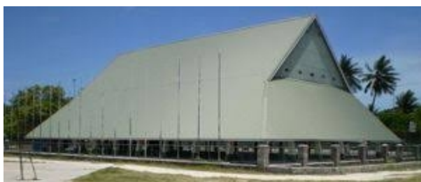
Figure 3. This is the Old and traditional look of Te Maneaba that can mostly seen in rural islands nowadays. This building made out of all local things which include lashing, wooden pegs, local strings, etc. 16
